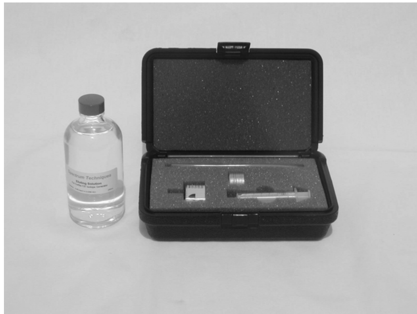
Figure 3: Isotope Generator to make Ba-137m from Cs-137
