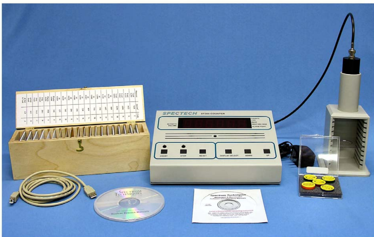
Figure 2: ST360 setup with sources and absorber kit.
